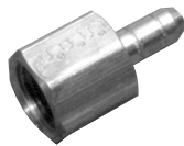
BRASS ADAPTOR • 1333 1/8" FPT TO 1/8" BARBED HOSE (May be used in place of brass base adaptor on manifold pressure switch)
