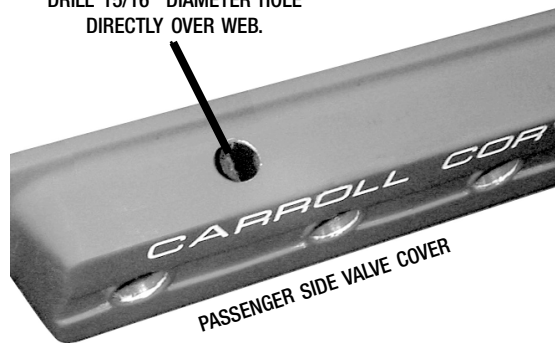
L98 CRANKCASE BREATHER INSTALLATION • 1069
