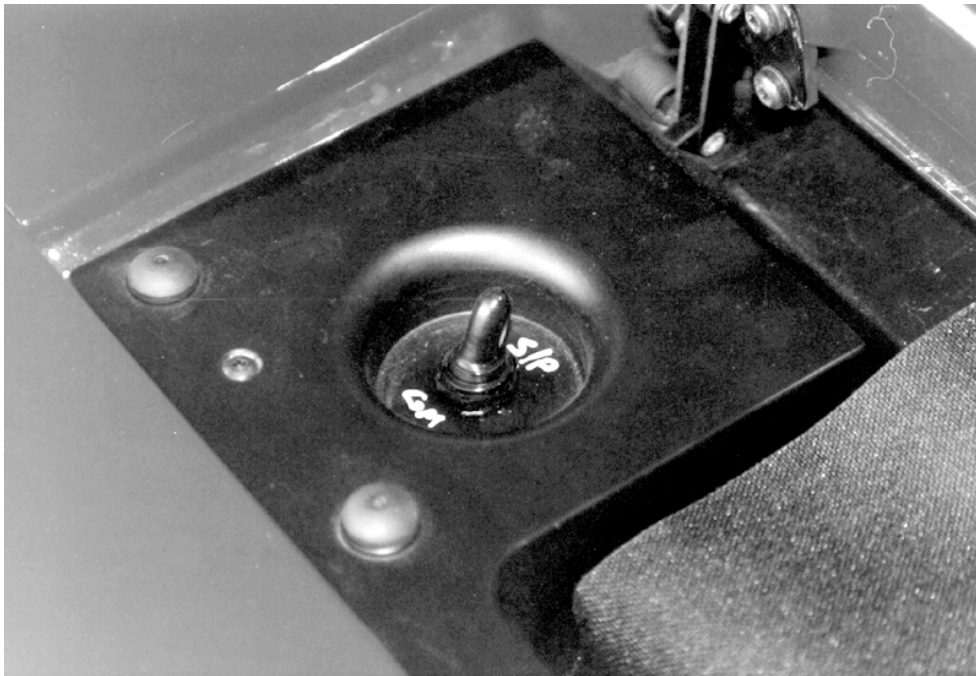
TOGGLE SWITCH LOCATED AT REAR OF VEHICLE ALLOWS FOR SELECTION OF STOCK GM MODE, OFF (VEHICLE THEFT) OR SUPERPUMPER.
