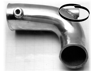
TYPICAL WELD-O-LET NOZZLE ADAPTOR ON VORTECH LT1 AIR DISCHARGE TUBE 1077
