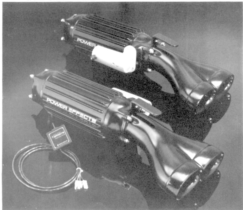
POWER CAPSULES w/cast aluminum tips & optional electronic remote tuning
