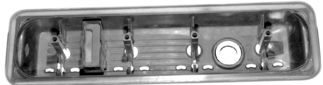
L98 VALVE COVERS AFTER MACHINING TO ACCEPT ROLLER ROCKERS
