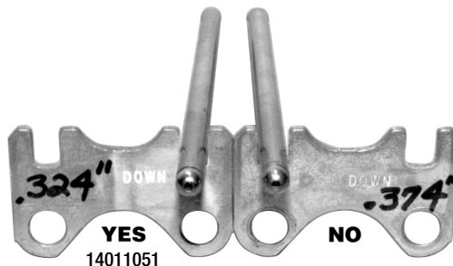
GM GUIDE PLATES – REQUIRED ON ALL GM ENGINES 1988 & NEWER WHEN INSTALLING ROLLER ROCKERS
