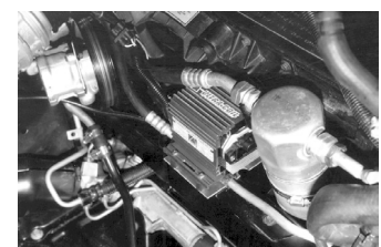
ULTRA HIGH ENERGY IGNITION COIL INSTALLATION ON AN LT1 VEHICLE
