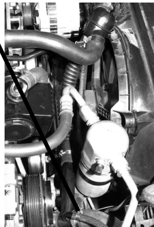
HEAVY DUTY EXTERNAL 3-WAY THERMOSTAT. Stock Thermostat Must Be Removed.
